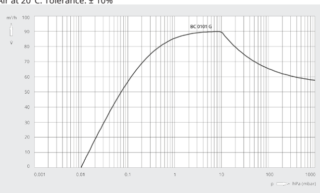
Pumping speed Air at 20°C. Tolerance: \pm 10\%
